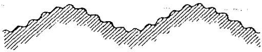
Figure 13.6 Composite rough-surface model of the sea with the small resonant water waves riding on top of the larger water waves, resulting in a tilting of the resonant waves from the horizontal.
